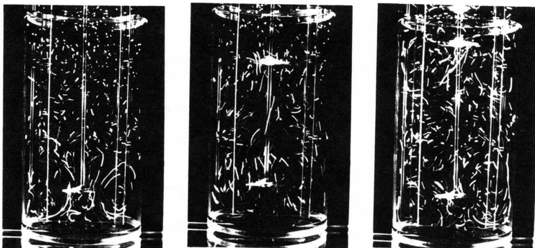
Figure 12a,b,c Streakline photographs for the impeller systems of Figure 10 and 11. The length of the streaks is proportional to the liquid velocity.
