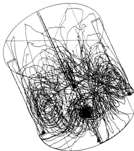
Figure 3 Trajectories of solid particles in the tank of Figure 2.
